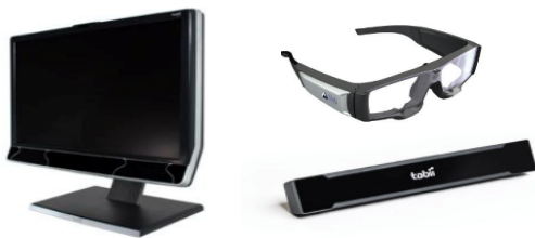
Figure 3. Basic equipment setup of an eye tracking laboratory space
